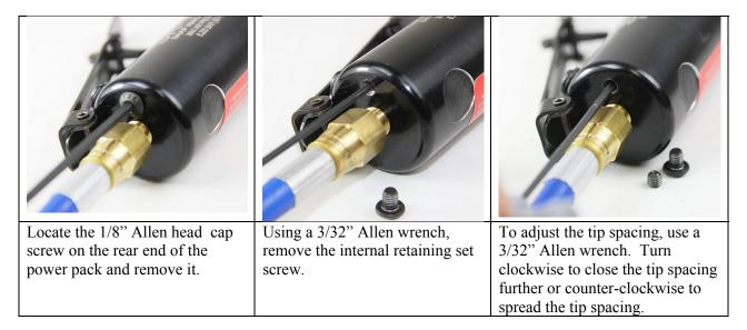
Once the tip spacing has been adjusted to match your specific snap ring, reinstall the retaining set screw and cap screw so lock in the tip spacing.
